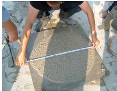
Picture 23 Slump flow measure method
