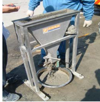
Picture 25 V shape flowing time test
