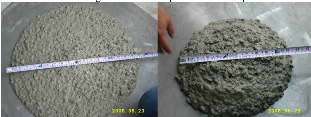
Picture 27 Slump flow difference between each batch
