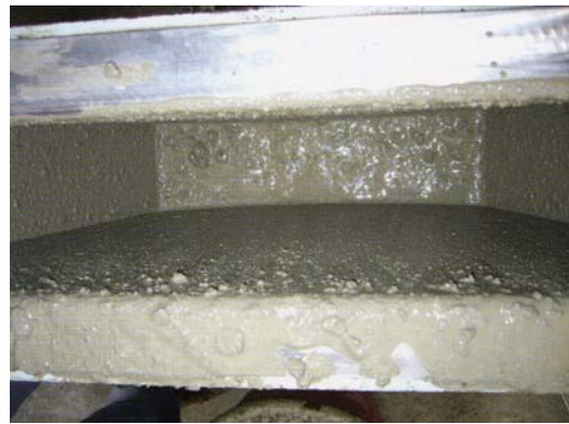
Picture 29 Mixture too cohesive increase flowing time
